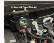
Universal Cowl Mount Installed: PAN040300-2 with 175-PO-150-2-PP
