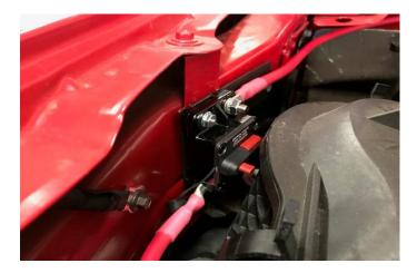
Completed installation. For illustration purposes only. Please verify cables are protected with loom and held securely and safely with ties.
