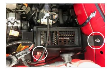
Completed installation. Verify that all wiring has been securely tied away from any edges of fuse panel.
