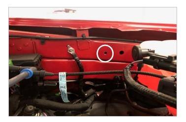
Factory unthreaded bung on inner fender will be used in conjunction with thread forming screw included.
