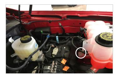
Lower mounting point utilizes factory coolant overflow mounting bolt.
