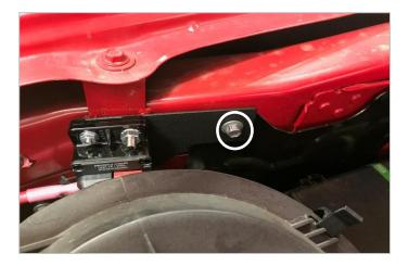
Factory thread forming screw will be used to mount circuit breaker to passenger side fender.
