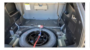
**Step 1.** Remove rear cargo floor panel and underlying foam filler panels. Foam panels are secured with M6 bolts and spacers.
