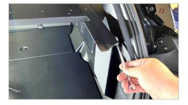
**Step 13.** Tighten all hardware. A ratcheting combination wrench eases tightening of side support and wing hardware.
