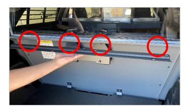
**Step 5.** Install forward support by removing nuts and washers from partition, placing support in place and replacing nuts and washers on partition. Hand tighten hardware
