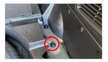
**Step 3.** Remove rear bolt from support bracket.
