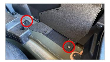
**Step 4.** Place support legs in position. With rear attachment hole aligned with threaded insert, replace rear support bracket bolt and tighten.
