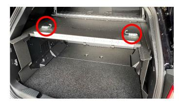
Completed installation with access door in raised position for improved access to lower cargo area.
