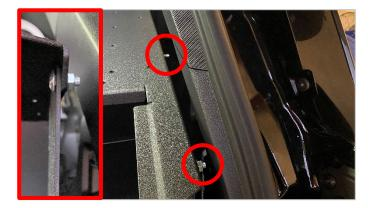
**Step 10.** Using two supplied carriage bolts and flange nuts, bolt shelf to side support surfaces (use rearmost hole only). One bolt per side, nuts toward outside. Forward hole will also be used for wing mounting.
