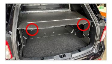
Completed installation with access door in closed position. Latches are released by simultaneously pulling inwards on each finger loop and lifting.
