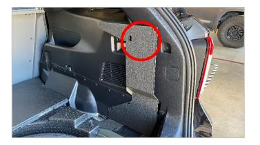
Cargo guard side supports are pre-punched for Sound Off Signal dome light models ECVDMLTST4 or ECVDMLTST4G. Passenger wing is pre-punched for Amerex model 862 fire extinguisher bracket.
