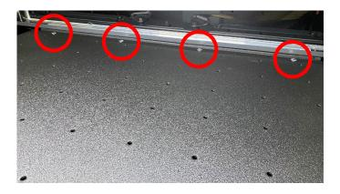
**Step 9.** Using four supplied carriage bolts and flange nuts, bolt shelf to forward support surface. Hand tighten only.
