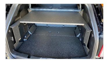
**Step 8.** Slide cargo guard into position and onto all three support surfaces.
