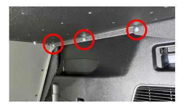
**Step 12.** Using supplied carriage bolts and flange nuts, bolt shelf to all three support surfaces, four on forward support and two on each side support.
