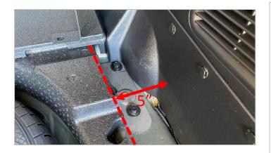
**Step 2.** Trim and reinstall both left and right forward underlying foam filler panels as shown. Trim foam pieces to approximately 5" from side trim panels. This will require removing about 4" of foam on passenger side and 2.75" on driver side.
