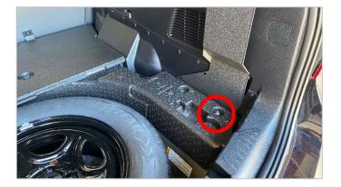
**Step 7.** Insert supplied 2 ¼" spacer & fender washer in hole in foam above threaded inserts and reinstall factory bolt. Note that spacer replaces factory spacer. Washer sits on top of spacer. Replace tire cover panel.
