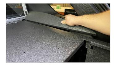
**Step 11.** Install side wings using six supplied carriage bolts and flange nuts. Three bolts per side, nuts toward outside.
